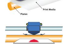
Step 1 - Built-in sensor detects thickness of print media
