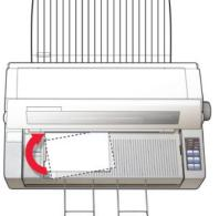
**Location-Free Paper Loading – Sheets** or forms can be hand-fed at virtually any point across the printer table; the ML8810 Series printer will sense the entry point and properly position the printhead.
